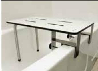
Swing down the legs 90 degrees until the "Locking Pin" snaps through the hole in the leg bracket, into its stopping position. The legs will be locked in their "down" position.
