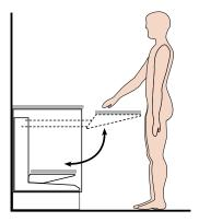
**UNILIFT** raises a panel from the bottom of a kitchen floor or wall cabinet to the desired working height. It can be used to lift food processors, microwaves or other household appliances.
