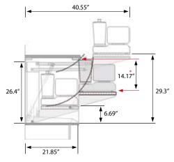
\* 14.17" cm maximum height of machine (at rear edge of support panel)
