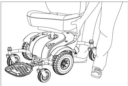
7. Take the controller and insert its square tube into the tube under the armrest.
