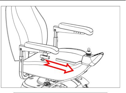
5. Pull the swivel lever up to unlock it and rotate the seat until it can be pulled up.
