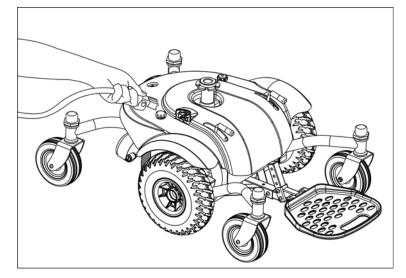
7. Release two star knobs from shroud. Lift the shroud straight up.
