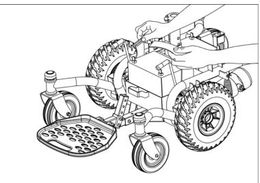
3. There are four connectors from main cable: Two black and red connectors are for batteries; two white connectors are for the motor.
