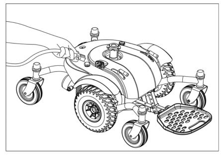
6. Lift the seat and pull the swivel lever up at the same time. Slide the bottom of the seat into the seat post.
