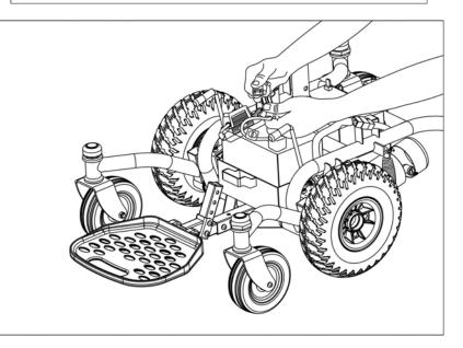
4. Carefully place the shroud, with the seat post and clutch levers fitting through their appropriate openings. Lock the shroud in place with the two star knobs.
