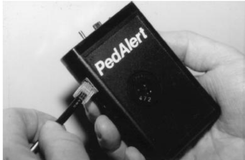
Figure 1. The wire needs to be firmly connected for proper operation.
