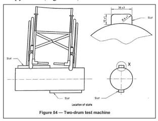
At Troy Technologies, we certify that our wheelchair can endure 100 hours on the accelerated fatigue two-drum test machine. That's more than double the national standard!
