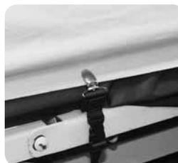
Fig. 3 - Sheet attachment clips (5750 only)
