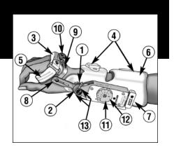
Position the red cable (1) around the top of the pulley. Push in and hold the black hinge knob (2). At the same time pull the
