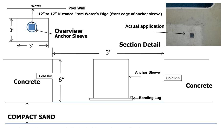
Front of Anchor Sleeve must be 12" to 17" from the water's edge Optimal placement is 14"
