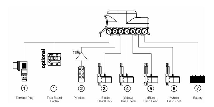
**Note:** The Foot Board Port of the MCL Control Box must have **either** a foot board control extension cable with a terminator plug or a foot board control cable **or** a terminator plug connected directly to the control box for any of the bed functions to operate. All beds are shipped from the factory with a terminating plug connected to the foot board port of the MCL Control Box or at the end of an extension cable plugged into the MCL Control Box.
