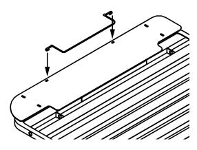
3. With the leg of each side of the End Mattress Retainer positioned in the ¼" holes, rotate the Retainer outward.
