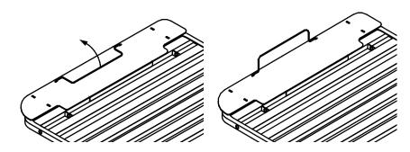
4. Place the mattress on the rib-deck sleep surface. Check that all edges of the mattress are within the Retainers. A slightly compressed fit is desired. Ensure that the Retainers hold the mattress securely to prevent mattress slippage during head and foot deck articulation.
