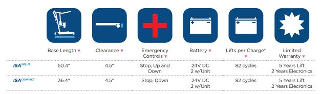
\*With battery charge between 100% to 50%
