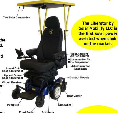
The Solar Companion still supplies solar power to the wheelchair even when it's in the down position.
