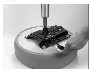
Insert the seat and cylinder assembly into the base and press firmly. Base should not detach from cylinder when stool is lifted. Then carefully sit down on the seat until the cylinder locks in place. The seat will be tipped 2 degrees toward the front. It is designed this way to relieve pressure on the thighs.
