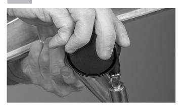
Invert seat and place on surface that will not damage the vinyl top. Place the button end of the adjustable cylinder into the opening of the seat tube. Press firmly. If you are having difficulty inserting the cylinder, use a rubber mallet to tap it gently into position. The cylinder should not fall out when the seat is inverted.
