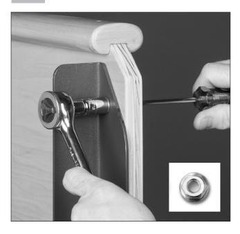
After the rear handrail has been secured, position the bolts on the right and left handrails so they line up with the holes on the uprights and secure with the remaining twelve (12) 7/16" washer nuts.
