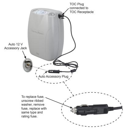
**NOTE:** The amount of power provided from the vehicle's DC electrical outlet is limited, the power available to charge the Battery is determined by the extra power available based on the operating demands of the TOC.
