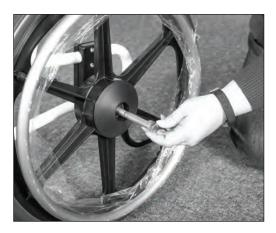
16. Place washer on bolt end to inside of wheel.
