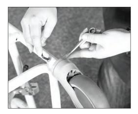
**10.** For shipping purposes, one wheel lock needs to be repositioned. Loosen the nut on the brake assembly mount just enough to turn the assembly upright using a wrench.
