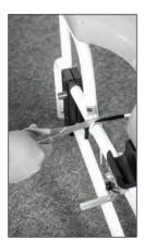
**3.** Set chair frame on its front end as shown. Loosen then remove the self-locking nut, plastic washer and machine screw that are in the chair frame where the anti-tippers will be inserted. If 4 casters were ordered, skip to step 6.
