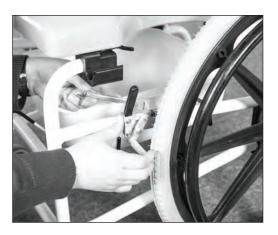
**22.** Loosen then remove the self-locking nut, plastic washer and machine screw that are in the chair frame where the back assembly will be attached.
