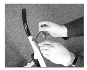
**6.** Set chair frame on its back end as shown. Loosen then remove the self-locking nut, plastic washer and machine screw that are in the chair frame where the casters will be inserted. If the 4 casters were ordered remove all 4 self-locking nuts, plastic washers and machine screws that are in the chair frame where the casters will be inserted.
