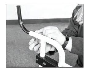
**5.** Use a wrench and hex key to tighten the rear anti-tippers into place.
