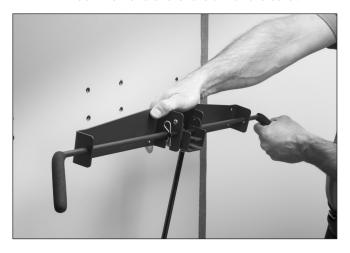
Secure the pneumatic cylinder's bracket to the backrest with the (8) eight 3/4" pan head screws.
