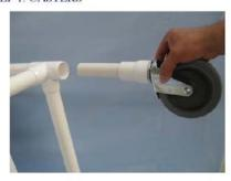
INSERT CASTER LEG STEMS INTO BASE SECTION.
