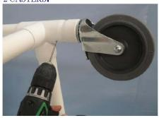
DRILL THROUGH LEG PIPES USING 1/8 DRILL BIT AND PILOT HOLES AS REFERENCE.
