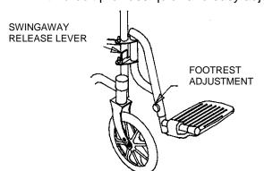
**Swingaway Footrests-** On wheelchairs equipped with swingaway footrests, activate the black swingaway release lever and the assembly will swing to the side. This feature permits easy entrance and exit to the chair.
