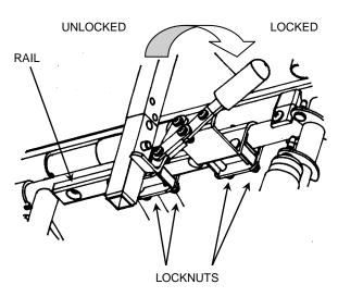
Reclining Back Models- Open wheelchair, install headrest and push bar shown below. Make sure spring buttons are fully extended through handles before use. This chair must never be used without both headrest and push bar installed. To adjust back angle, grasp both pusher handles securely and pull both release levers at the same time. Gently lower or raise the back to the desired height. then release the levers.
