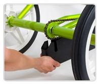
Detach the back of the bottom cover by pushing down.
