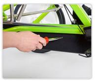
Use a Phillips screwdriver to remove the screw in the side of the chain guard.
