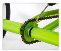
Place two drops of oil on the rear axle on either side of the toothed gear sprocket where the plastic chain guard rests to prevent squeaking.
