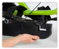
Remove the front of the bottom cover by pushing it forward, then pulling down.
