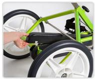
Remove the top cover of the chain guard by lifting at the back.
