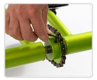
Tighten the rear sprocket screw with the 5/32" hex-head wrench. The gear sprocket should be centered left-to-right on the rear axle when tightened.
