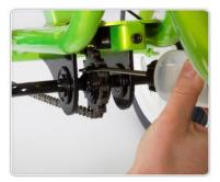
Place two drops of oil on either side of the front gear sprocket.
