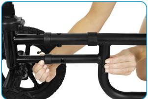
3. Insert a Screw Knob (F) into the top of the frame above the locking pins and twist until fully tightened to secure the scooter wheelbase.
