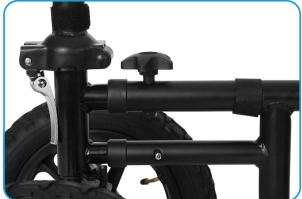
4. Pull the silver tension lever assembly up until the lever and the spring bolt are vertical and parallel to the steering column socket.
