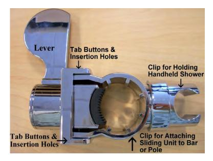
Separate the clip piece from the lever piece by depressing both sides of the clip piece at the same time so the tab buttons will come free of the insertion holes.
