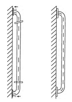
2) Connect the Slide Bar Bracket to the Slide Bar. See detailed photo instructions if needed.
