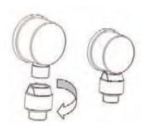
5) Connect the Hose with the Vacuum Breaker as shown in the drawing.
