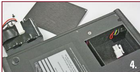
1. Using a small Phillips screw driver remove the battery cover.
