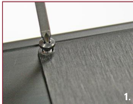
1. Using a small Phillips screw driver remove the battery cover.
