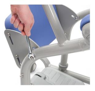
To adjust the height of the Knee Pad, loosen the four screws with an allen key (as shown below). Reposition the Knee Pad to the required height then retighten using the allen key.
