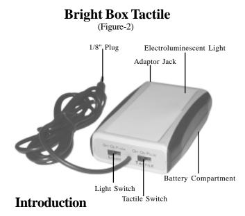
Your *Bright Box Tactile* switch was designed with a largedisplay visual feedback and with tactile feedback that are activated when the user presses the top surface of the switch. The visual feedback is comprised of a large, flat electroluminescent lamp (EL) that glows a bright bluish, green color. The tactile feedback is a vibration much like that of a cell phone or pager.
