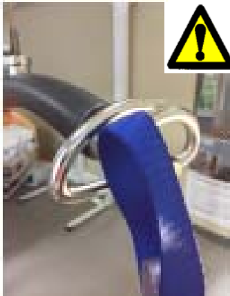
Load applied. The sling loop begins to slide off the hook.
