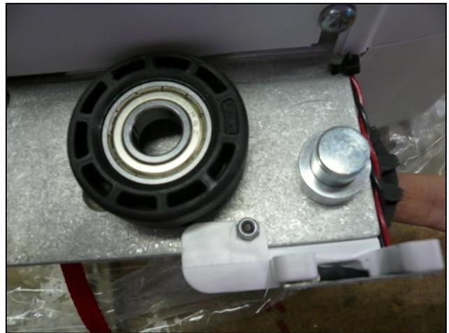
Remove & replace wheel from shaft
