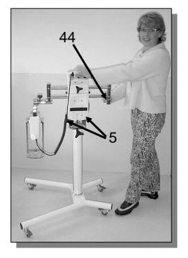
For easy transport, the unit features 4 wheels with brakes and the sliding motor mount bar (44) that also functions as a handle.
