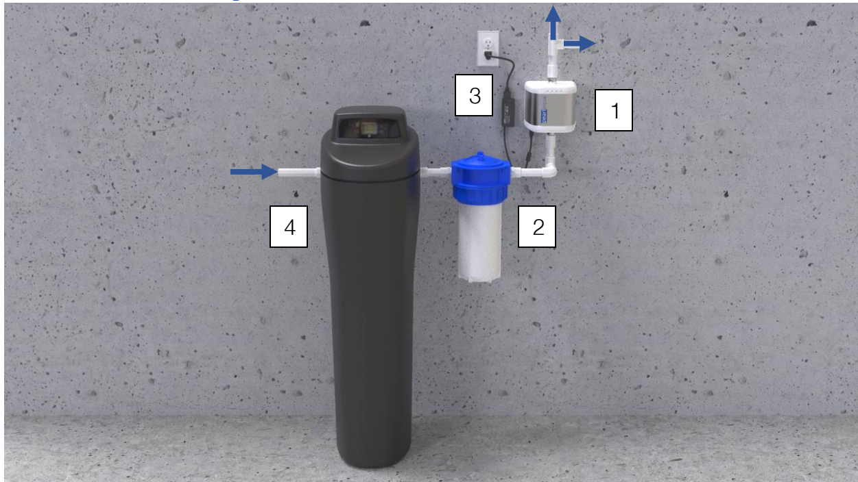
Figure 3-3: Typical diagram of PearlAqua Deca installation
