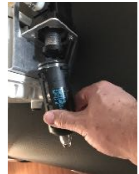
Put the black bulb back on pushing up and giving it a quarter turn to make sure it is securely connected.
