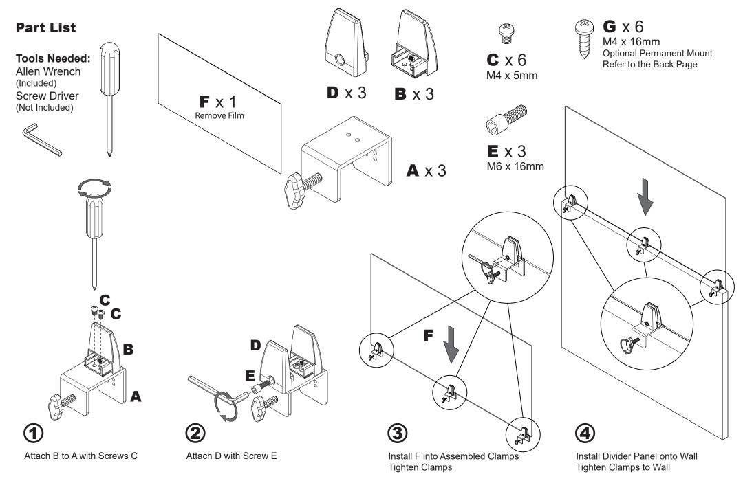
DIVWT 3 Clamp Wall Divider Panel Assembly Guide Optional Permanent Mount
