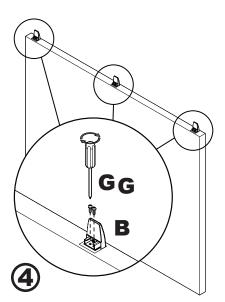
Remove and Disassemble the Panel Assembly. Place Part B on the Wall in the Outline Location and Secure with Screws G.
