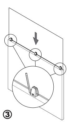
With Assistance - Place the Panel Assembly on the Wall and Outline the Clamps with a Pencil.
