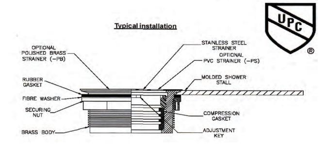
APFDR, is for use only with ABS/PVC pipe connections and not recommended for cast iron piping.
