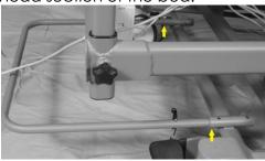
Align holes in Wall Guard with receiving tube and place pins through the holes on
