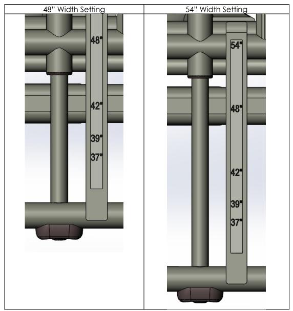
**NOTE:** This bed can accommodate 39", 42", 48" and 54" mattresses. The appropriate mattress **MUST** be used, such as a Drive Medical Pressure Reduction Mattress for each width setting.
