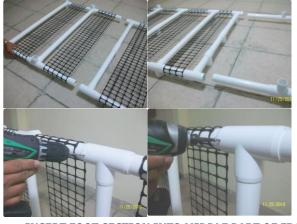
INSERT FOOT SECTION INTO MIDDLE PART OF FRAME
