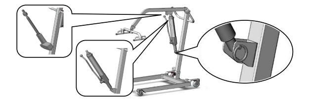
**A.** Attach bottom piston of either the Hydraulic Pump or Actuator by sliding it between the Mast brackets. Secure with steel pin and key ring.
