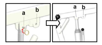
*ii.* The Electric Actuator shall be installed at position: **b**
