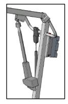
After installing the Hydraulic Cylinder, the assembly of the Hydraulic powered lift is complete. The following assembly instructions apply to PL400EL and Electric Upgrade Kit users only.
