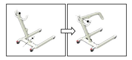
C. Attach the Hydraulic Pump and then Spreader Bar
