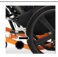
The mag wheels feature 3 mounting positions for forward adjustment to accommodate individual needs for stability and maneuverability.
