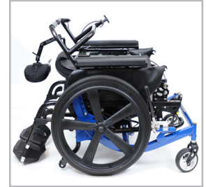
Back canes fold down for easy vehicle loading.
