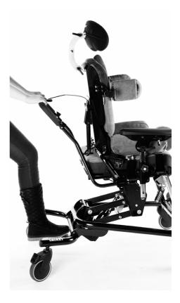
You can carry out this adjustment with the user in the chair. To adjust the height of the hi-low chassis use a pump action on the foot lever at the rear of the chassis whilst holding the push handle. Once you remove your foot from the pedal the seat will be fixed at the chosen height.
