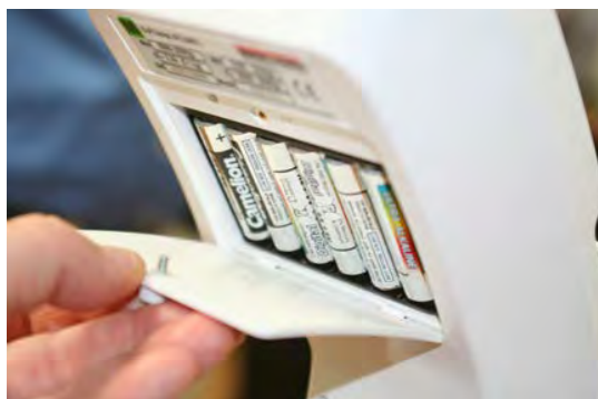
Figure 2-8. Batteries in Battery Chamber
