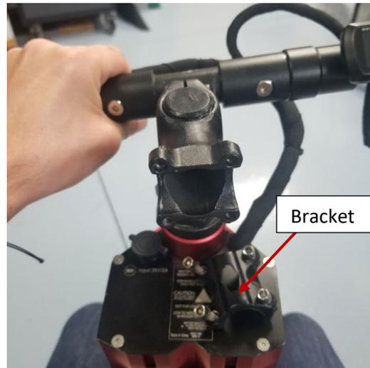
2. Then loosen the two screws that clamp the handle bar stem to the steering column using a 5mm hex key. Only loosen the stem until it is able to rotate.
