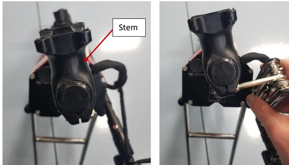
4. Place the handle bars back on along with the bracket and start by hand tightening the four screws to get the threads started. Then tighten the screws in a pattern using the multitool so all screws will be tightened down evenly.
