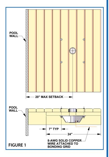
\*NOTE: Bond anchor to bonding grid with 8-AWG solid copper wire per local electrical codes as required.
