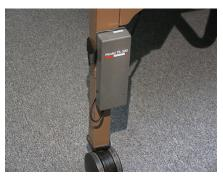
The LT-900 Long Range Transmitter has a switch on the side of the unit to turn the transmitter on for instant or delayed operation or off to allow the caregiver to work with a patient and not have the alarm sound.
