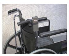
The LT-900 Long Range Transmitter has a switch on the side of the unit to turn the transmitter on for instant or delayed operation or off to allow the caregiver to work with a patient and not have the alarm sound.
