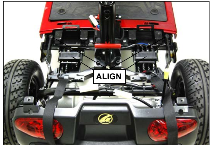
FIGURE 21. CORRECT FRAME ALIGNMENT
