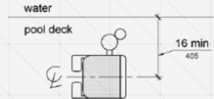
Figure 1009.2.2 Pool Lift Seat Location
