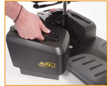
Step 2: Pull out the battery pack!
