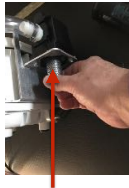
Unscrew the silver filter piece. Screw on the new silver filter
