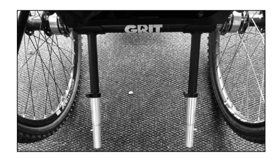
The Anti-Tip Bars are shipped at GRIT's recommended length. The length can be adjusted to make the bars more secure or more permissive. **To adjust the bar length:**
