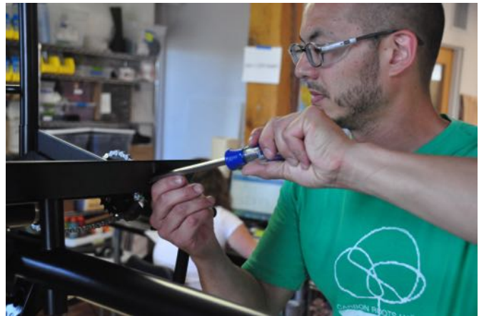
(d) Use a #3 (or any available) Philips screwdriver to tighten the setscrews until the desired chain tension is reached.
