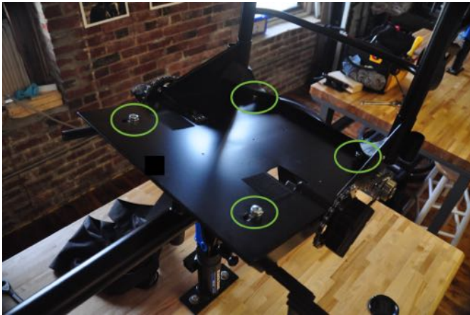
(a) Four bolts must be loosened (and later retightened) to slide the seat.
