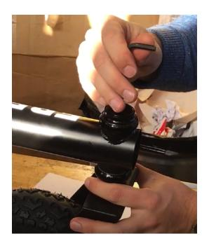
2) Use an Allen key to loosen the headset (the pieces that secure the front fork to the boom of the chair). Remove the headset bolt. Slide the fork out of the boom of the chair. Place the headset pieces in a small bag and set the bag and the front wheel/fork aside for now.
