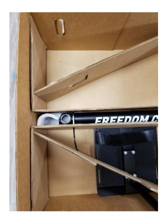
12) Feed a zip-tie through the first triangular insert, under the boom, through the second triangular insert, and back. This zip-tie helps prevent the chair from moving around in the box. Add paper or foam dunnage in front of the boom.
