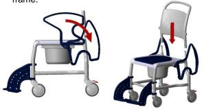
Swivel the armrests forwards until they click into the slots of the backrest and the locking pins click into the lower frame. Be sure they are securely in place.
